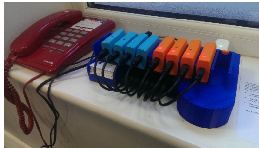
The Complete WayWard Tracking System in situ with eight tracking boxes.
